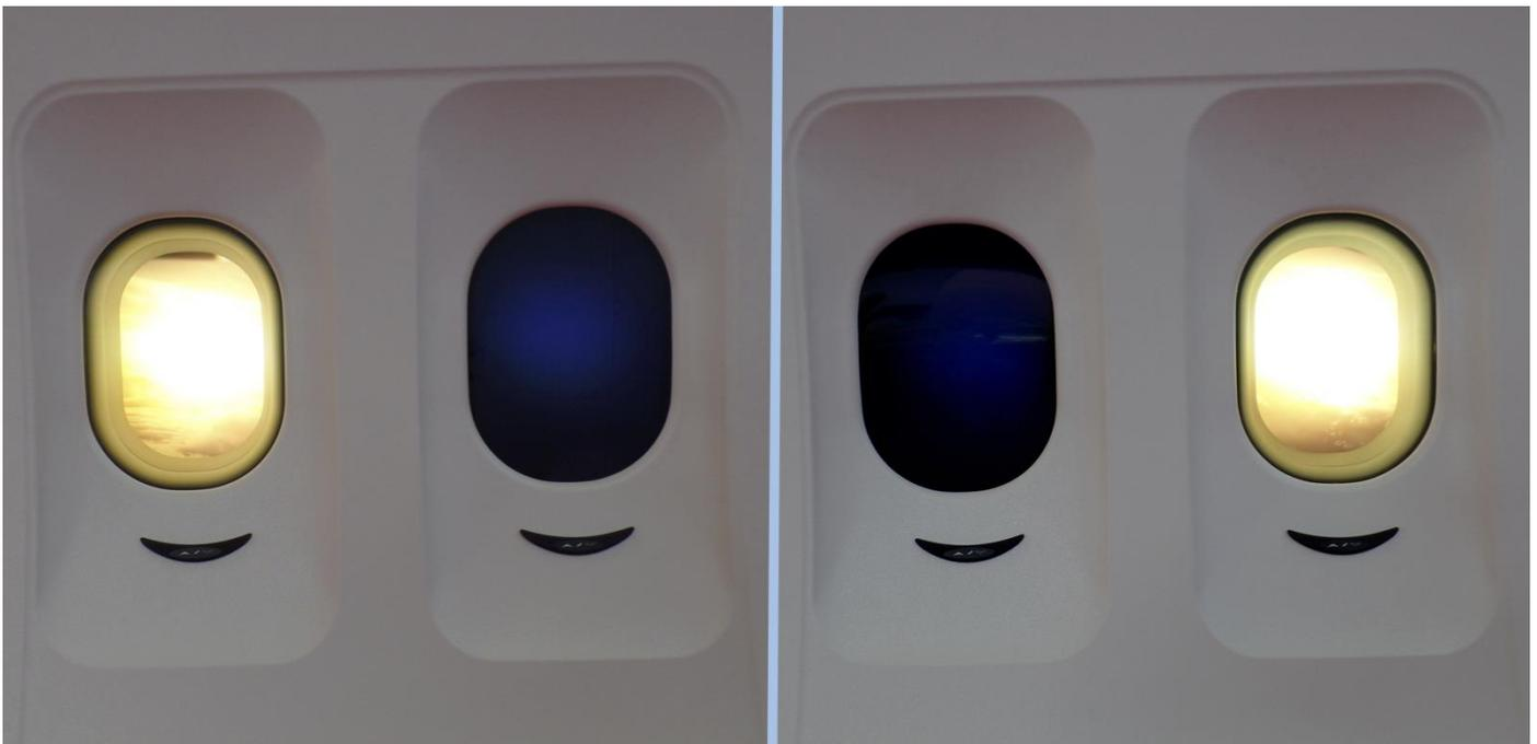
*At 2016 MRO Europe, Fokker Services had the world premier of Element EDW – electronically dimmable windows for in-service commercial airliners. It has been designed for both single-aisle and dual-aisle aircraft.*
