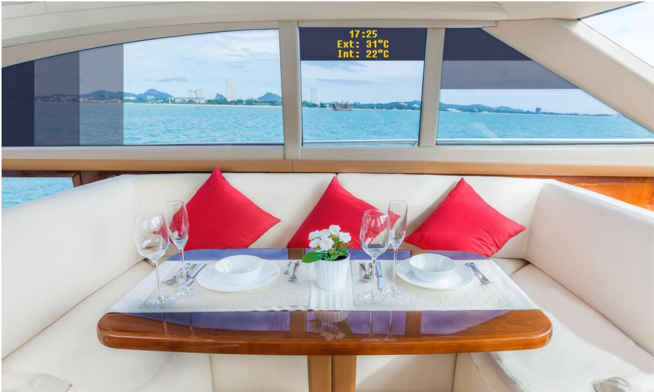
*Vision Systems' SPD-SmartGlass electronically dimmable windows (EDWs) feature electroluminescent technology to display information, and the ability to control the level of tint in different zones.*
