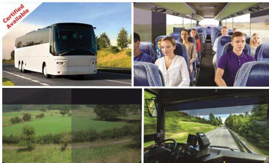
*Vision Systems’ electronically dimmable windows and windshields, using Research Frontiers SPD-SmartGlass technology, improving the passenger experience onboard motorcoaches.*
