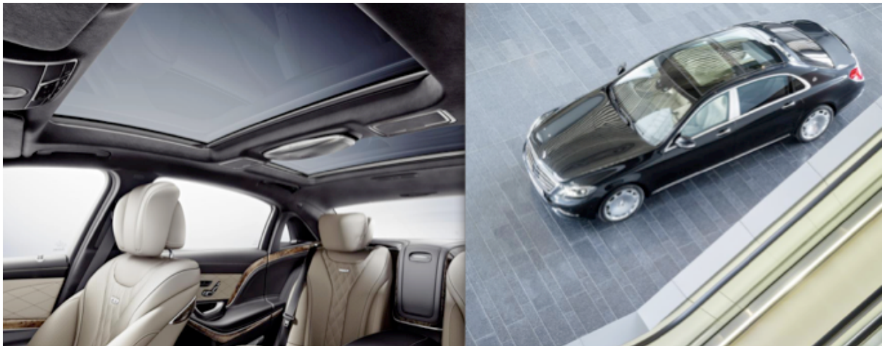
The first-ever sliding MAGIC SKY CONTROL roof using SPD-SmartGlass technology from Research Frontiers offered on the Mercedes-Maybach S 600.
