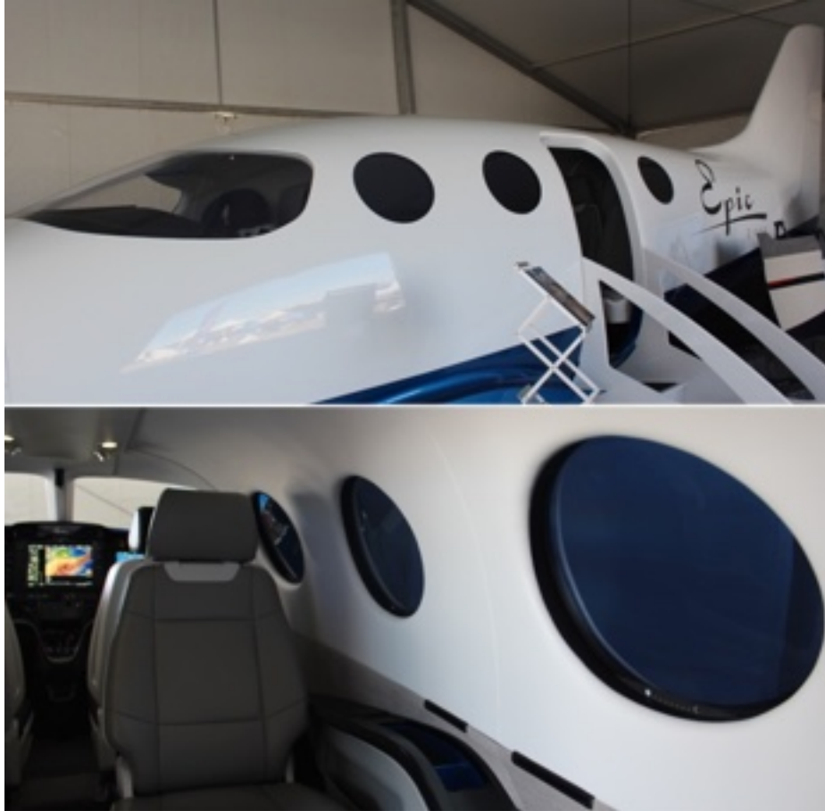
Epic Aircraft E1000 mockup with SPD-Smart EDWs, at 2015 NBAA in Las Vegas, Nevada
