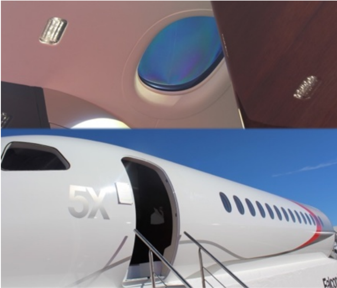
Dassault Falcon 5X with SPD-Smart skylight, at 2015 NBAA in Las Vegas, Nevada
