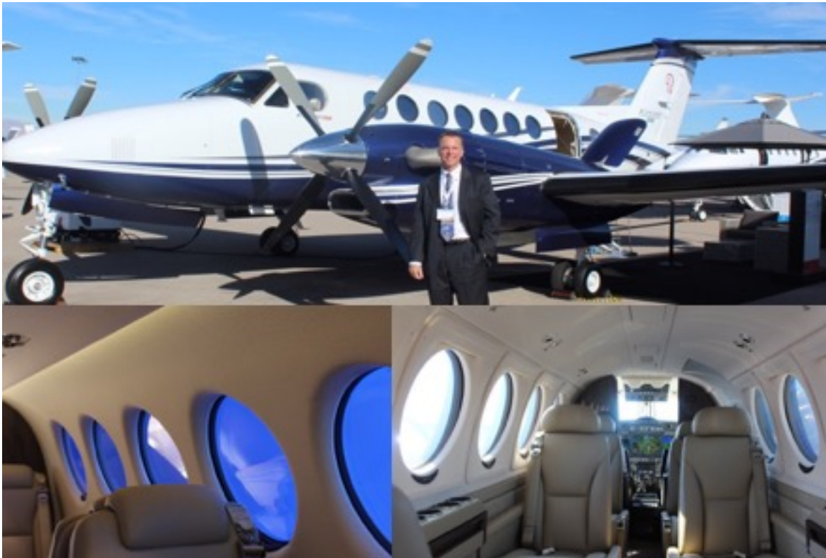
Textron Beechcraft King Air 350i and King Air 250, with SPD-Smart EDWs, at 2015 NBAA in Las Vegas, Nevada
