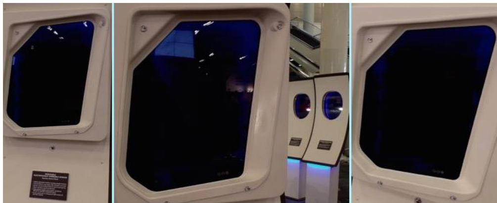
Vision Systems SPD “Nuance Smart Shade” Electronically Dimmable Window for cockpit side windows.
